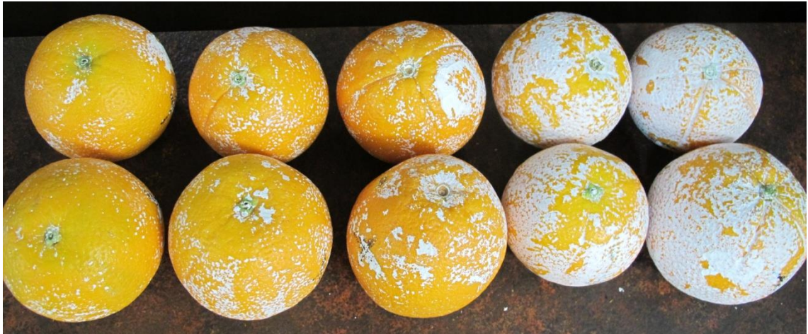
Figure 10. These oranges pictured indicate a range of paint removal from one pass under a citrus HPW. Clearly there are efficacy issues with this unit.
