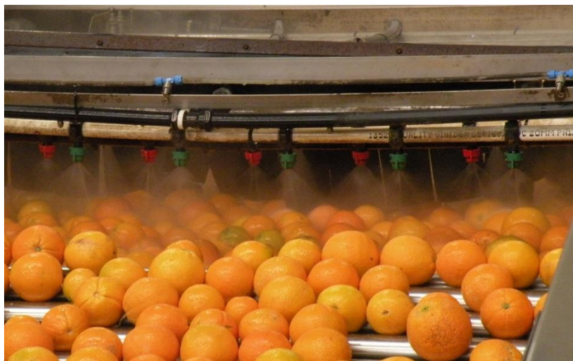
Figure 13. Oranges exposed to a clean water rinse after HPW.
