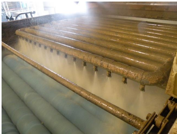
Figure 4. (A) An example of organic matter build up on the gantry of a HPW.
