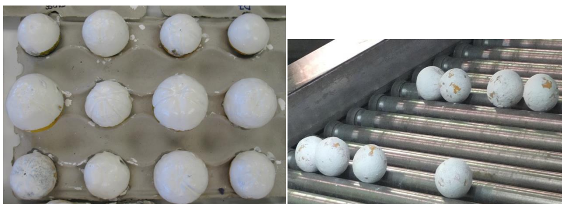
Figure 9. Oranges dipped in PVA/Surround® mixture and dried and then run over the washer.
