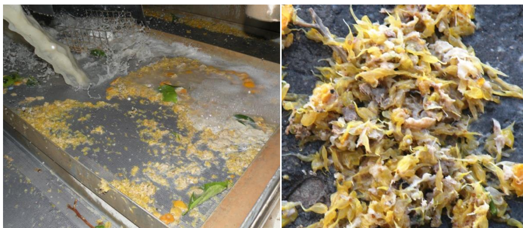
Figure 14. An example of a flat mesh type filter system in a high pressure citrus washer (A) and the nature of the material that blocks the filters (B) which is mostly fruit pulp from rotten fruit.
