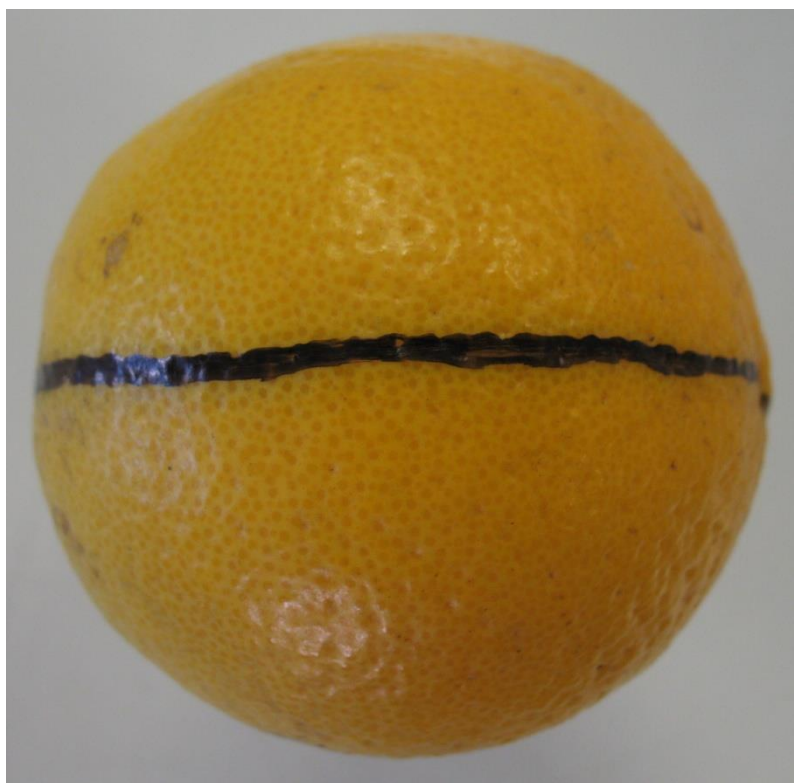
Figure 8. Medium sized orange with black line marked across/around it for counting rotations on the brush bed.
