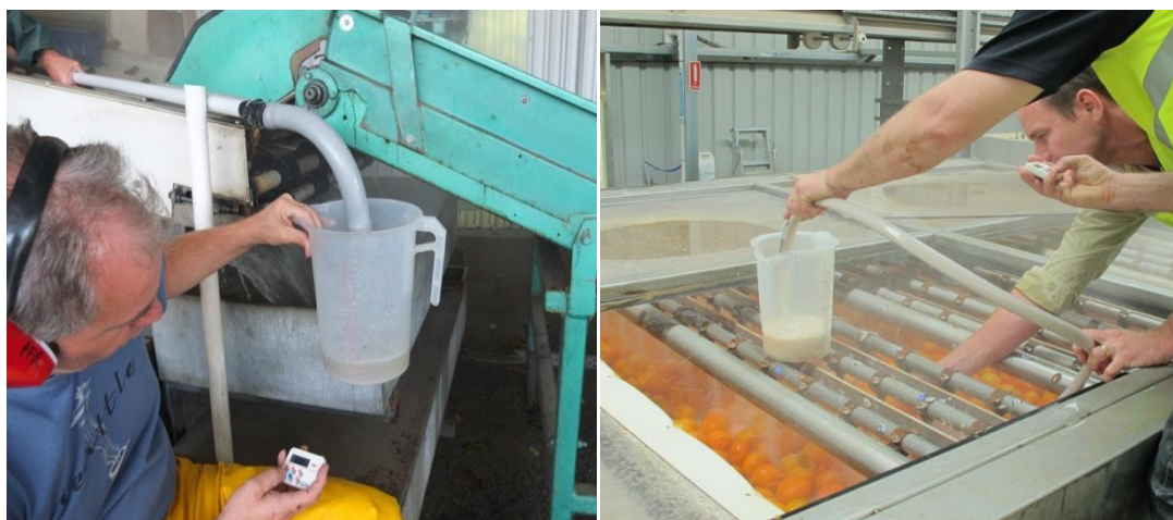
Figure 7. Measuring flow rate. Time to fill to 1.5 L is measured for each nozzle. Hose should be fitted before turning the water on.
