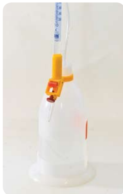
Auto-fill burette – simply squeeze the bottle to fill the burette.
